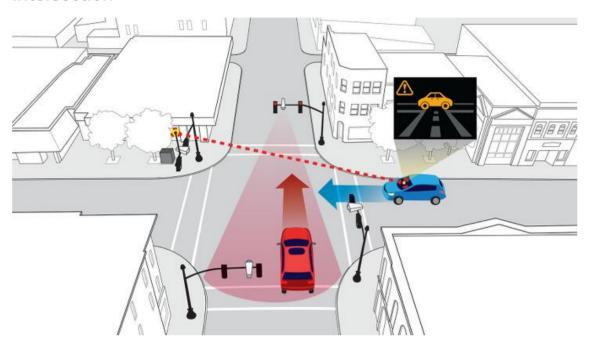
Target Vehicle approaching from oncoming direction while Ego vehicle is taking a left turn
